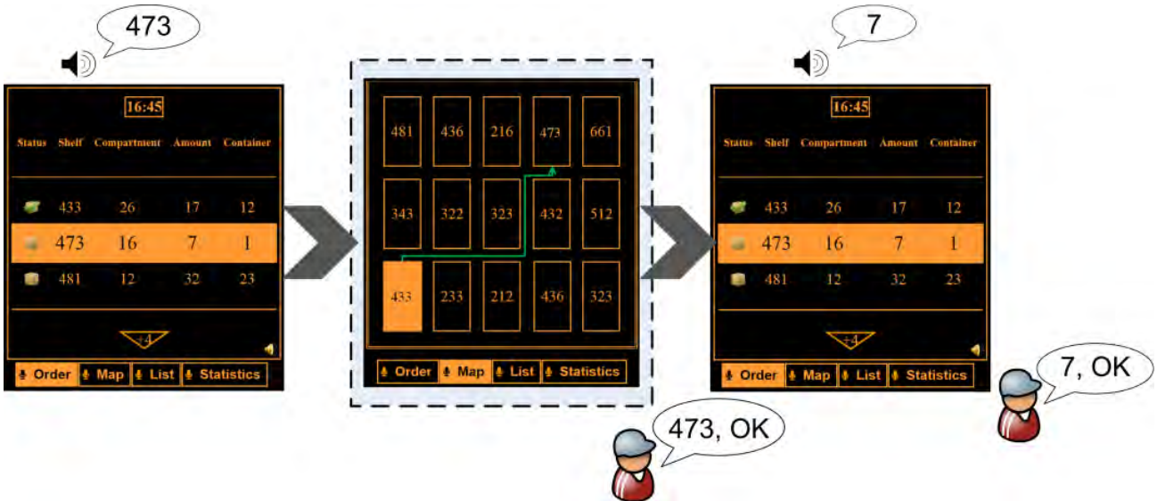
Fig. 3. Basic interaction flow with adaptation: the execution of the rule for an experienced picker omits the appearance of the Map view (dotted line)
