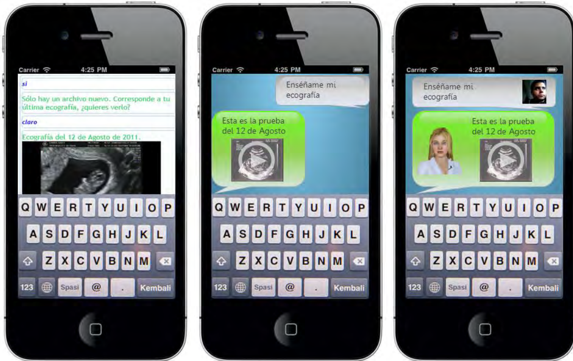
Figure 5 Different approaches for a Virtual Help Assistant on a touchscreen smartphone: Left: Direct rendering of the desktop system. Middle: Adaptation using chatting with text messages. Right: Adaptation preserving the ECA functionality.
