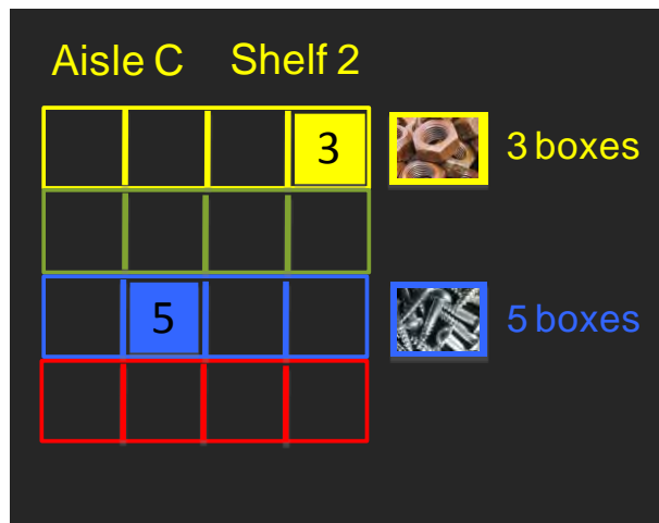
Figure 16: Graphical user interface for the wearable computer to directly support the task of picking.
