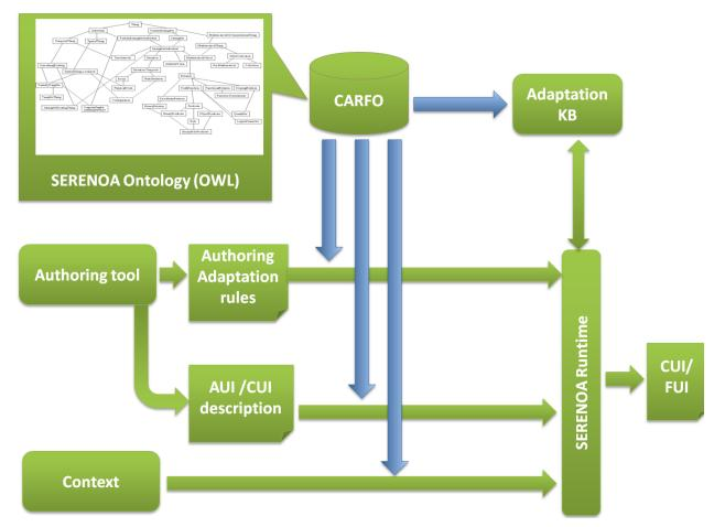
Figure 5: Adaptation data flow. Blue lines mean concept definitions and green lines are exchanged streams of data
