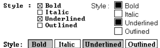
Figure 2. The AIO check box in different environments : Check box in Ms-Windows, XmToggleButton in OSF/Motif, BoxArray in Garnet.
