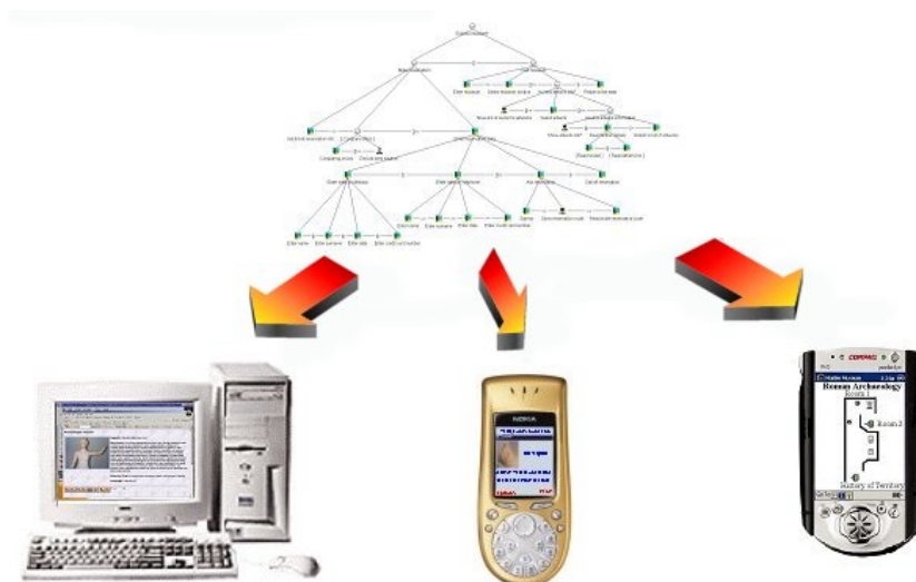
Figure 6: Deriving multiple user interfaces from a single task model
