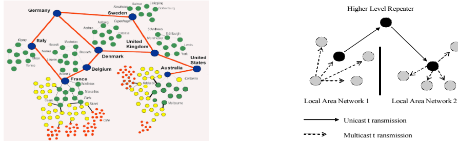
Fig. 4. An Hybrid P2P hierarchical architecture inspired from [13]. a) An example of network topology at the planet level. b) A mix of multicast transmissions at the local level, and unicast transmissions at the global level. Grey circles denote contextors, whereas black circles represent repeaters.
