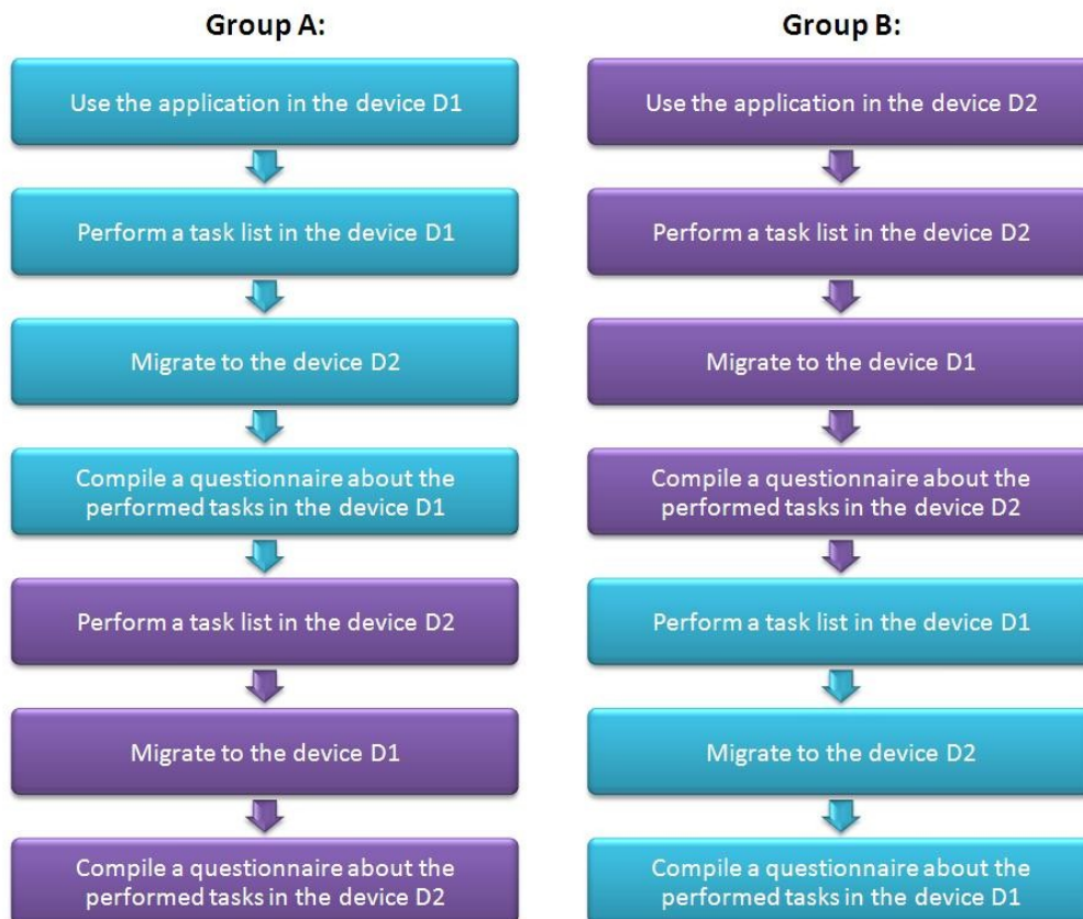
Figure 4: Method used in order to avoid bias problems during comparative usability tests
