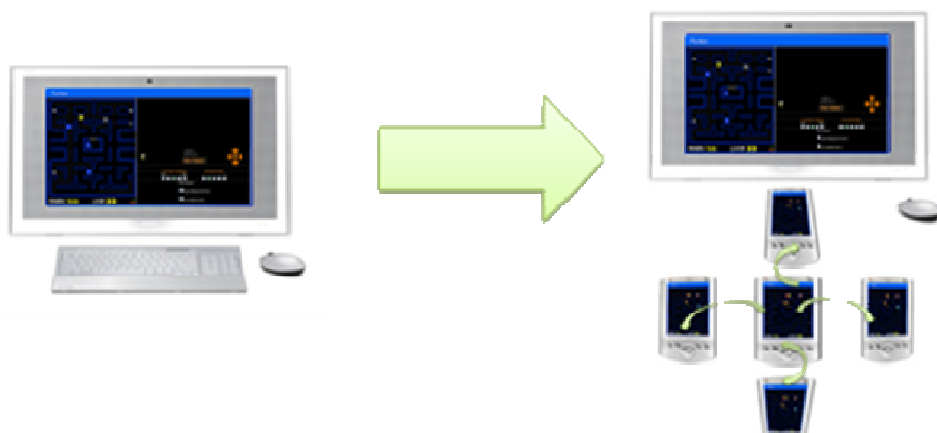
Figure 3: The control of the PacMan is migrated from the keyboard of the PC to a PDA with an accelerometer. After migration the PacMan can be steered by tilting the PDA. The GUI stays at the display of the PC.
